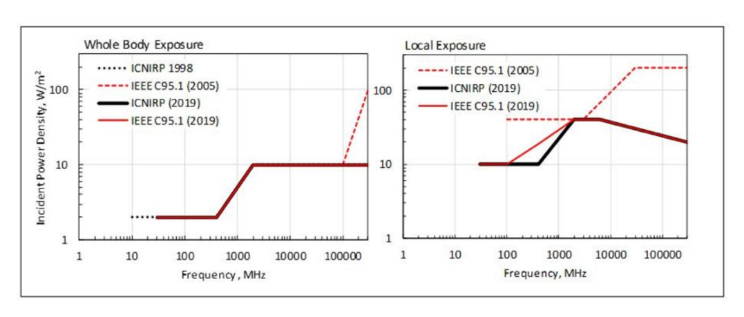
Figure 1 Exposure reference levels for general public in ICNIRP and IEEE.
